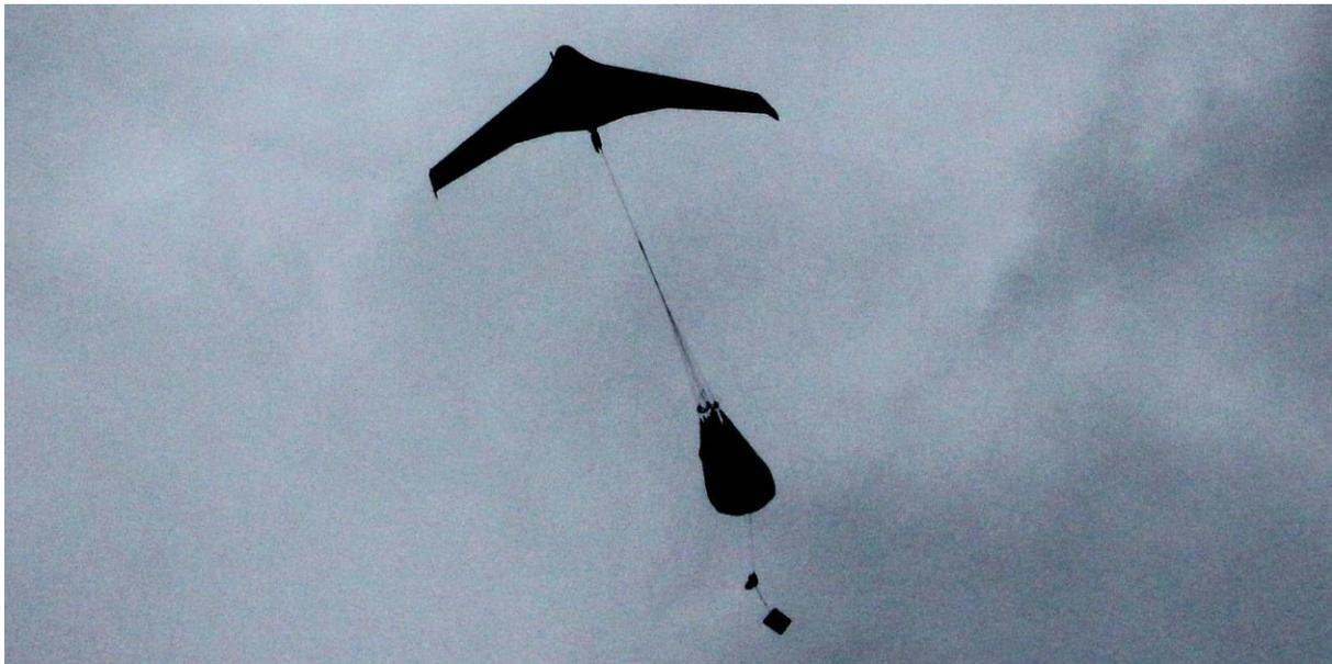
C-Astral Bramor RPAS (Remotely Piloted Aircraft System) deploying its parachute for a landing
