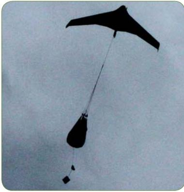
Fig. 3: The C-Astral Bramor UAV during the initial deployment of its landing parachute.
