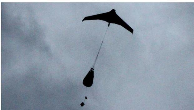
Figure 4: The C-Astral Bramor RPAS during the initial deployment of its landing parachute.
