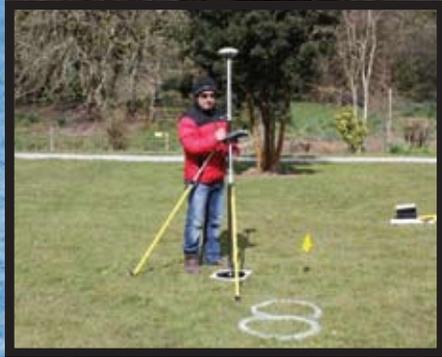
**INSET, TOP:** Ground control station and check point targets.
