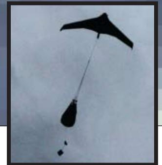
**INSET, ABOVE:** The C-Astral Bramor UAS during the initial deployment of its landing parachute.
