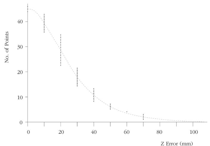
The distribution of vertical errors derived from the figures in the table showing the dataset of measured errors.
