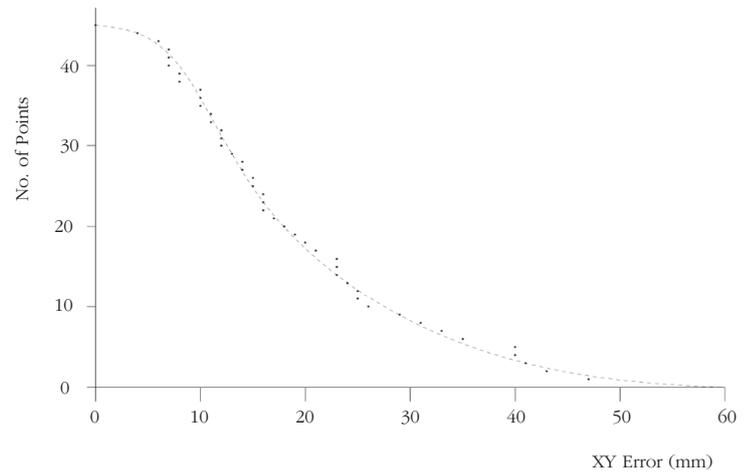
The planimetric distribution of errors derived from the figures in the table showing the dataset of measured errors.
