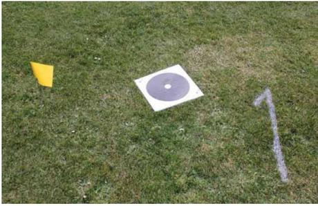
Ground control station and check point targets.
