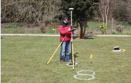
The stabilised Trimble GoeXR Network RTK GNSS used to get the coordinates of the target centres.
